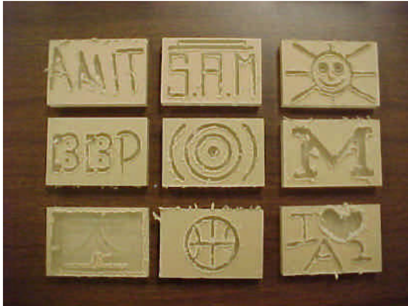
Figure 5: Some of the student designs that are machined
